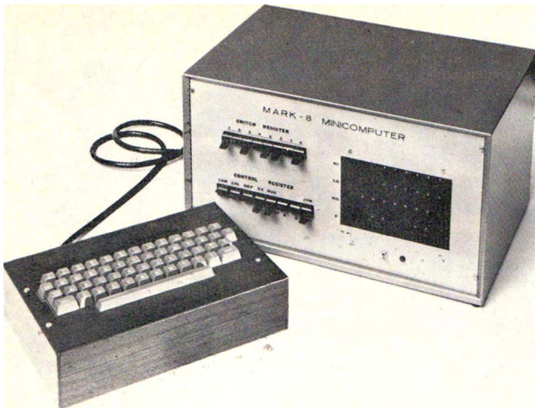
COMPUTER WITH ASCII KEYBOARD makes a complete working computer system. You can use the computer without the keyboard, but it is more difficult.
